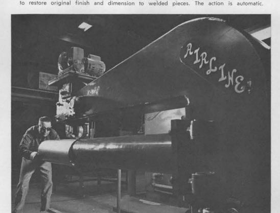
AFTER WELDING CYLINDER, Leslie Cox places it on planishing roll machine. Metal expands
